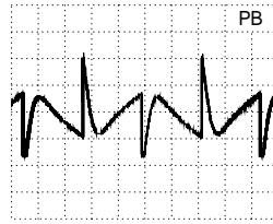
DC, 500mV/Div, 500µs/Div Connector 1930-(4) ⑤⑤
